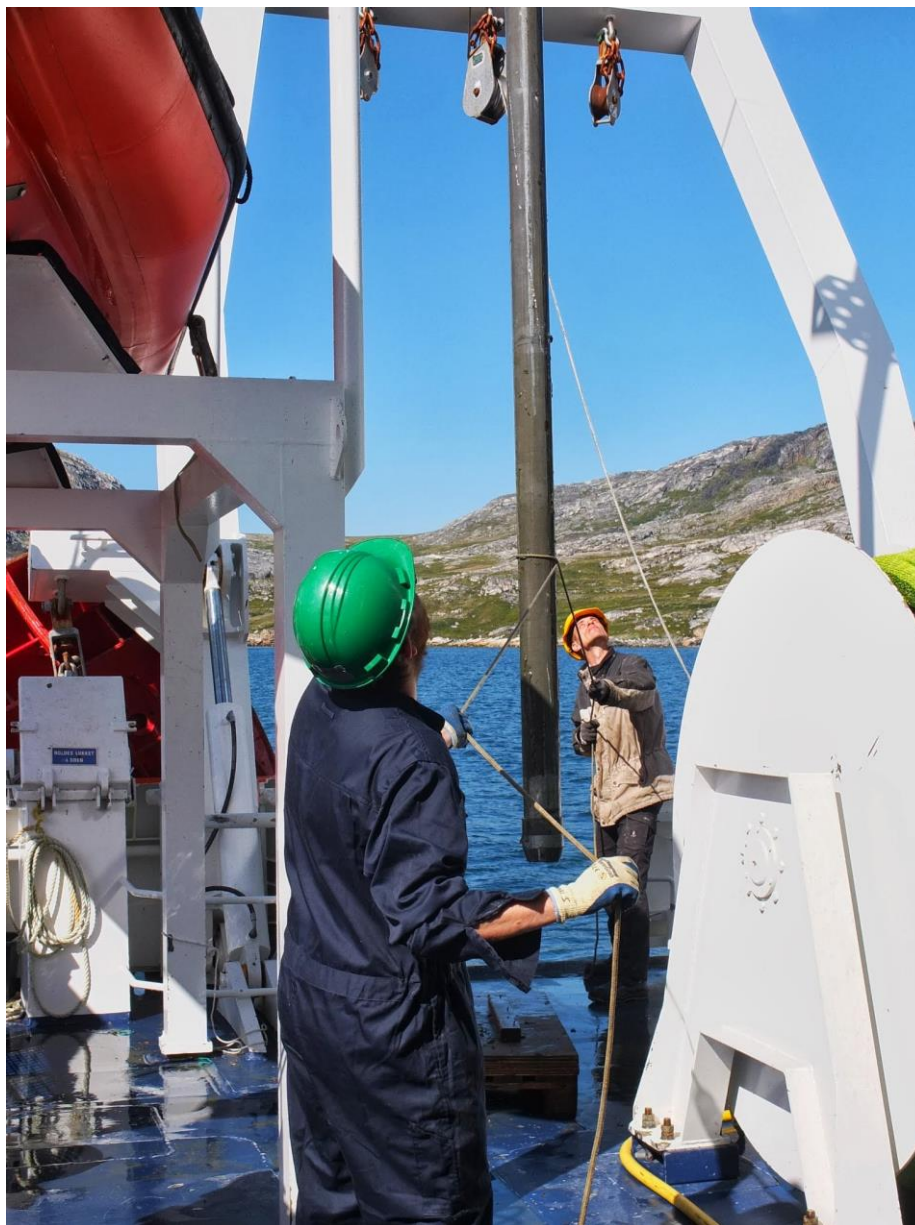
Figure 2. For long sediment coring, a 6-m gravity corer deployed using the ship's main winch and A-frame. (Photo: Christof Pearce).
