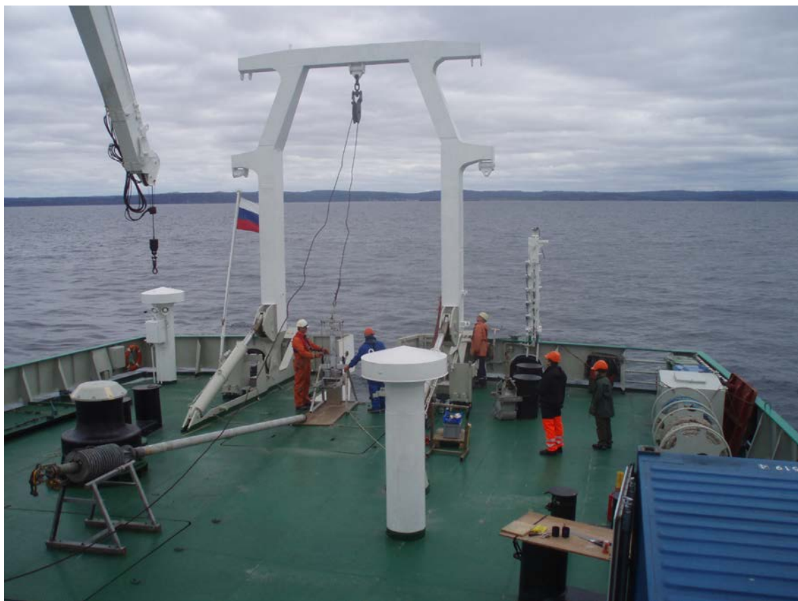
Figure1. For sediment sampling, a 6-m gravity corer and a box corer from GEUS were deployed using the ship's main winch.
